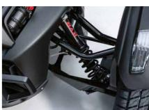
**FULL KYB HPG SHOCKS** Front and rear KYB HPG shocks with remote
